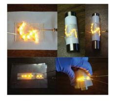
A highly conductive polyurethane (PU)-based adhesive is developed by generating and sintering silver nanoparticles in situ during the curing of silver/PU composites. With the high conductivity, mechanical compliance, good adhesion, and compatibility with various flexible substrates, the PU-based adhesive is promising in support of various advanced interconnection techniques for flexible electronics, including flip-chip and 3D integration.
